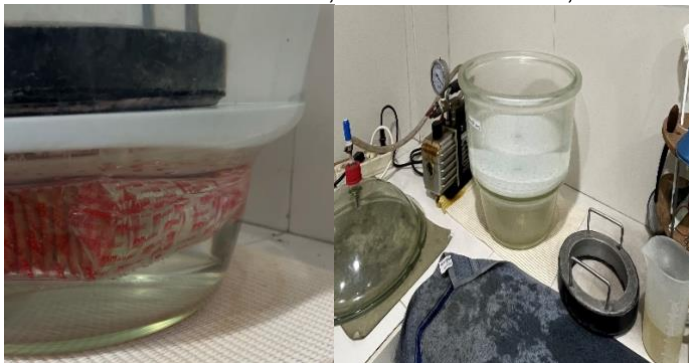
Figure 1 Vacuum test used for leakage detection of primary packaging sample
